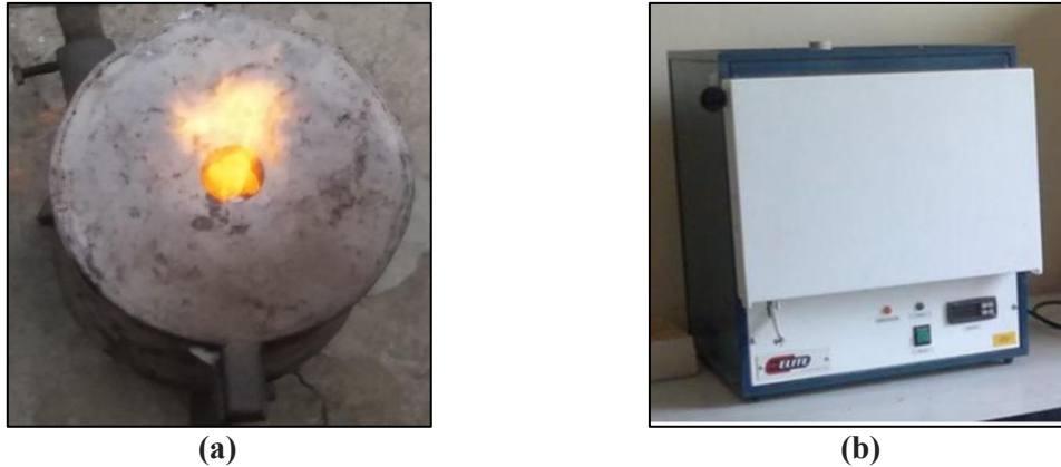
Fig. 3: The used furnaces (a) the gas furnace for manufacturing the cast alloys (Al-Nima, 2021) and (b) the employed electric furnace for corrosions testing (Al-Nima, 2021; Ikhdhayyir and Hammoud, 2022).
