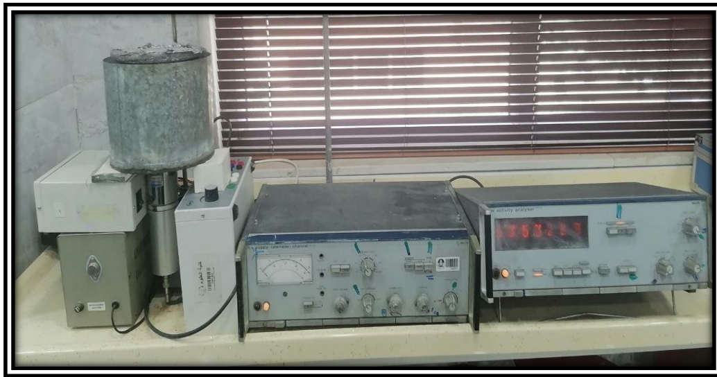
Fig. 3: Soil erosion measurement system using Cesium-137 (Cs-137)
