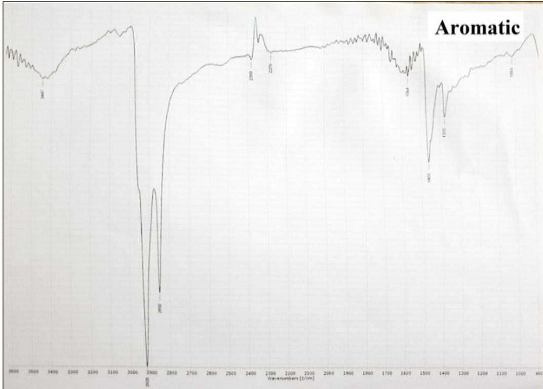
**Fig. 8: IR spectrum for aromatic part**
