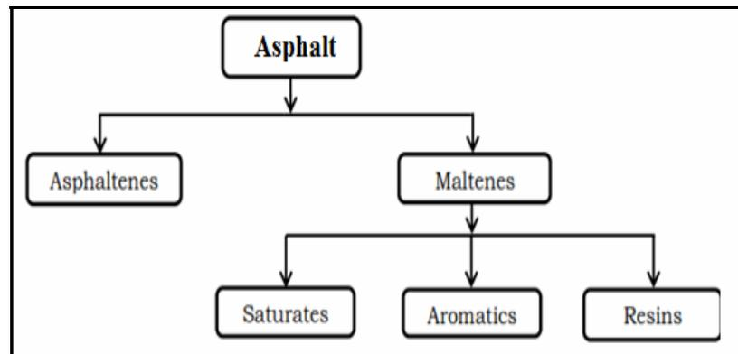
**Fig. 1: (SARA) Parts separated from asphalt Materials**
