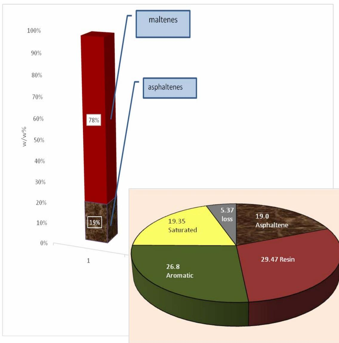
**Fig. 4: Fractions of asphalt**
