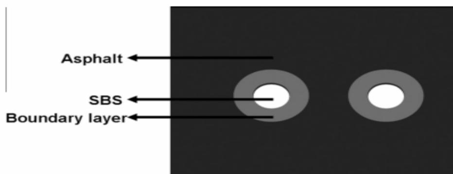
**Fig. 3: Modification mechanism of SBS modified asphalt**
