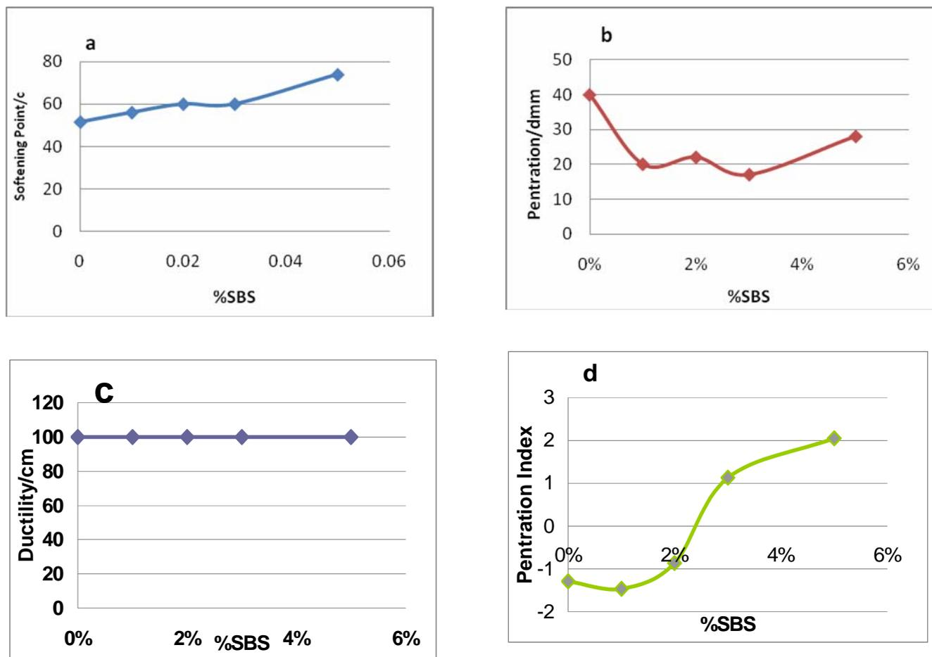
**Fig. 9: physical properties after adding the polymer to the asphalt (a: softening point, b: penetration at 25 °C, c: ductility (cm), d: Penetration index)**
