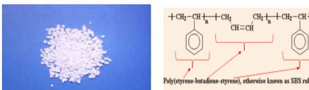
**Fig. 2: A; Image of material SBS , B; Chemical formula SBS****Preparation of Sample**
