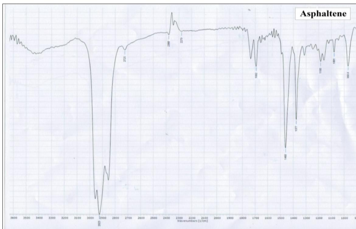
**Fig. 5: IR spectrum for asphaltene**
