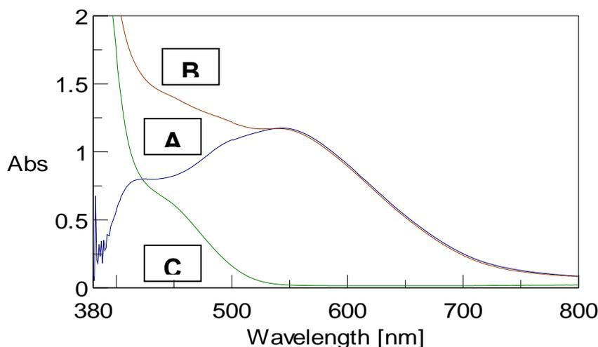
**Fig. 2: Absorption spectra of 25 µg CAP / 10 ml treated according to the recommended procedure and measured against (A) reagent blank, (B) ethanol and (C) reagent blank measured against ethanol.**
