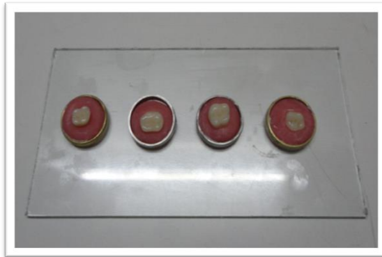
Figure (1): The acrylic teeth were embedded in auto polymerizing acrylic resin using a metallic ring mold.
