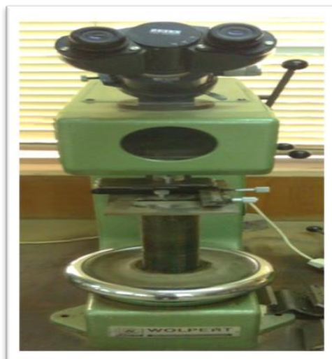
Figure (3): WOLPERT Vickers microhardness tester.
