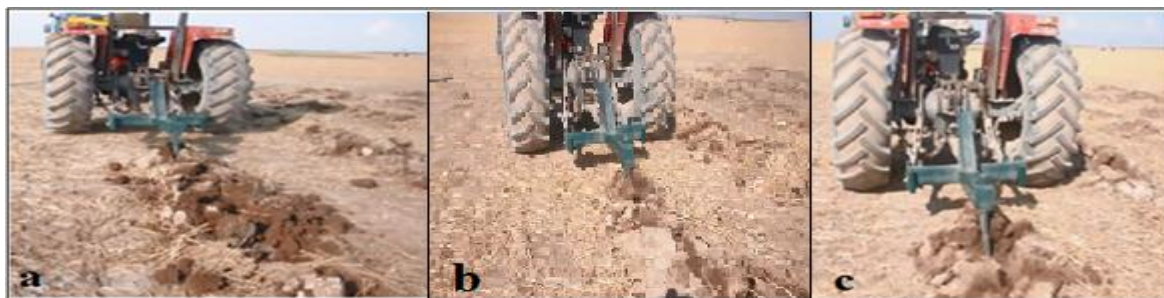
Figure (3): The tillage result using three types of shanks in the field. (a) bent shank (b)curved shank (c) straight shank
