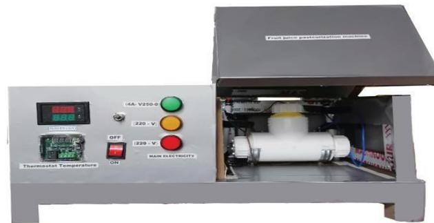
Figure 2: Manufactured batch Ohmic heating apparatus Ohmic heating of the orange juice.
