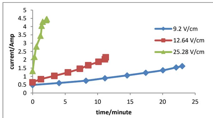
Figure 4: time and current profiles as affected by different voltage gradients (9.20, 12.64, 25.28 V/cm).
