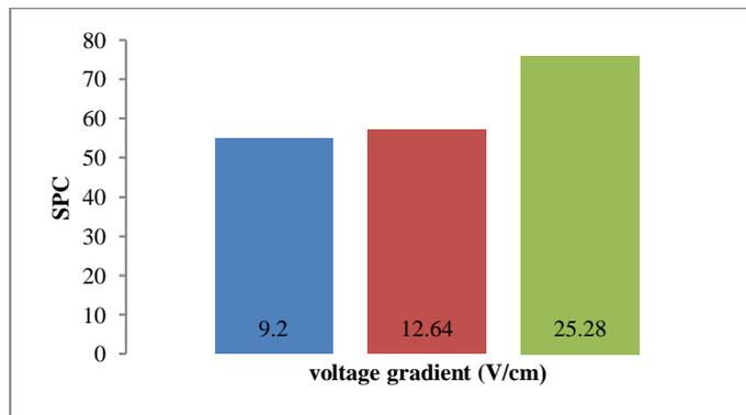
Figure 7: SPC of the manufactured Ohmic heating device at different voltage gradients.
