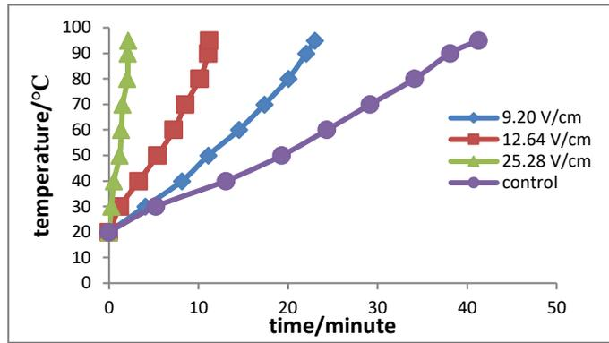
Figure 3: Curves of Ohmic heating time versus temperature of orange juice at different voltage gradients (9.20, 12.64, 25.28 V/cm).
