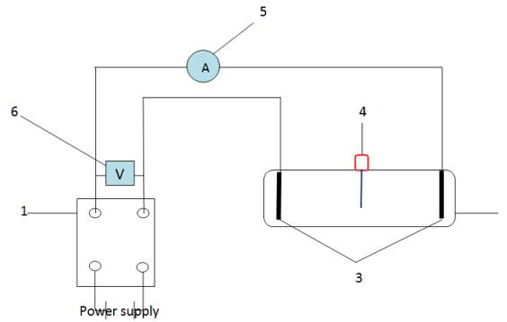
Figure 1: The scale in the laboratory Experimental system for ohmic heating. 1, Ohmic heating tube; 2, electrodes; 4, thermocouple; 5, Ampere digital screen; 6, Voltage transformer.
