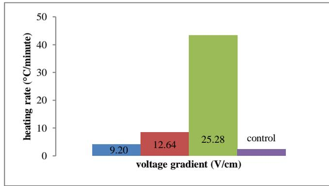
Figure 8: The heating rate at different voltage gradients.
