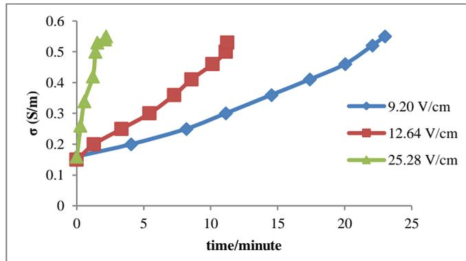
Figure 5: Electrical conductivity depending on-time processing according to voltage gradients (9.20, 12.64, 25.28 V/cm).
