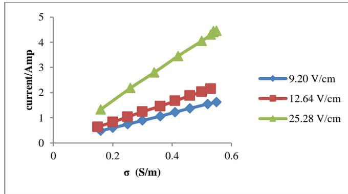
Figure 6: current profile changes with increasing electrical conductivity at different voltage gradients.
