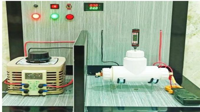
Figure (2): batch type ohmic heating equipment
