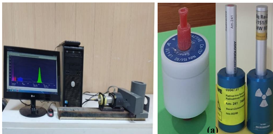
Figure 1. (a) Gamma-ray spectroscopy system used to study the radiation protection standards for glass samples. (b) – Standard sources of Cs-137, Am-241, and Ra-226.
