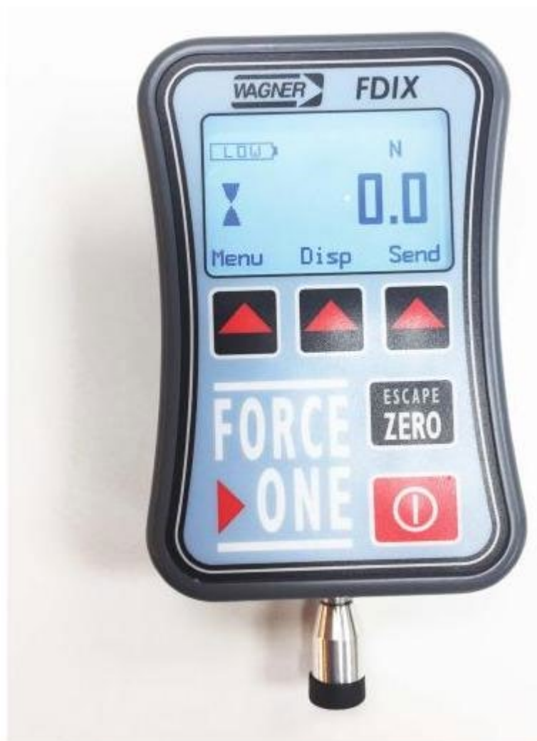
Figure 5. Hand held Digital Algometer (Wagner Pain Test™ - Model FPIX): a Digital device that give accurate pressure/force readings.
