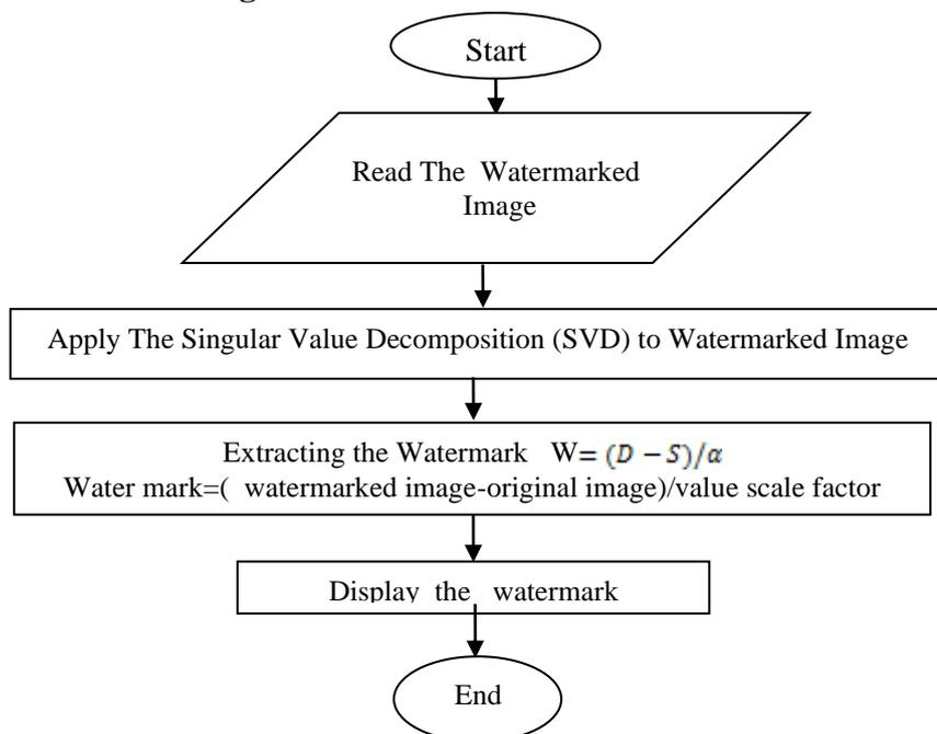
**Figure 7: Flow chart of the extraction process**
