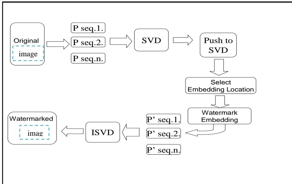
Figure 4: Diagram of Watermark Embedding
