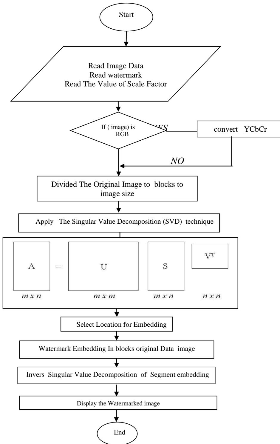
Figure 5: Flow Chart of the Embedding Process
