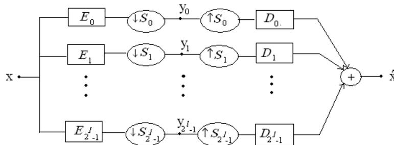
Figure (9). The multichannel view of an  $l$ -level tree-structured DFB
