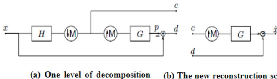
(a) One level of decomposition (b) The new reconstruction scheme
