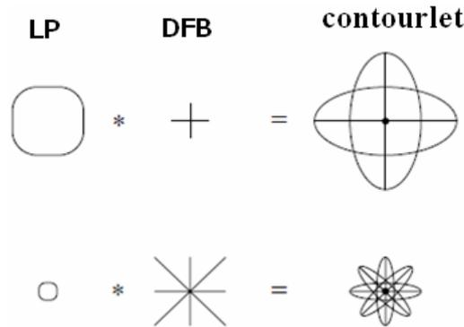
**Figure (7).** Illustration of the contourlet basis images that satisfy the curve scaling relation. From the upper line to the lower line, the scale is reduced by four while the number of directions is doubled.
