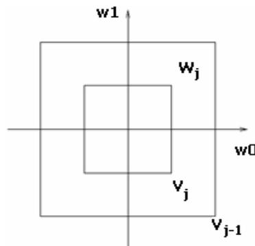
**Figure (8).** Multiscale subspaces generated by the Laplacian pyramid.
