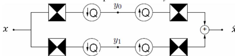
**Figure (5).** Two-dimensional spectrum partition using quincunx filter banks with fan filters. The black regions represent the ideal frequency supports of each filter. Q is a quincunx sampling matrix
