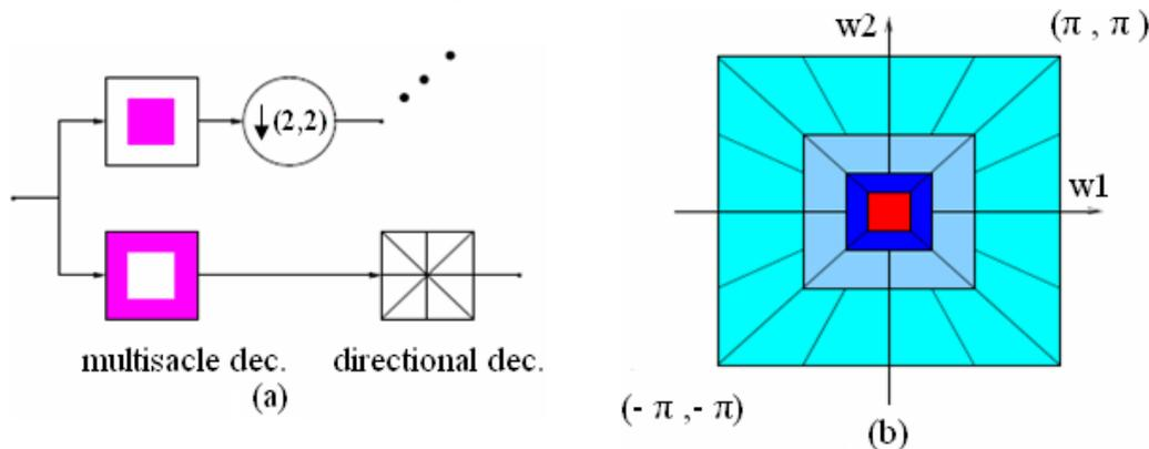
Figure (2). The Original Contourlet Transform. (A) Block Diagram. (B) Resulting Frequency Division
