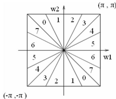
**Figure (4).** Directional filter bank. Frequency partitioning where  $l = 3$  and there are  $2^3 = 8$  real wedge-shaped frequency bands. Sub-bands 0–3 correspond to the *mostly horizontal* directions, while sub bands 4–7 correspond to the *mostly vertical* directions
