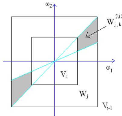
**Figure (11).** Multiscale and Multidirectional Subspaces Generated by the Transform this is Illustrated on 2-D Spectrum Decomposition
