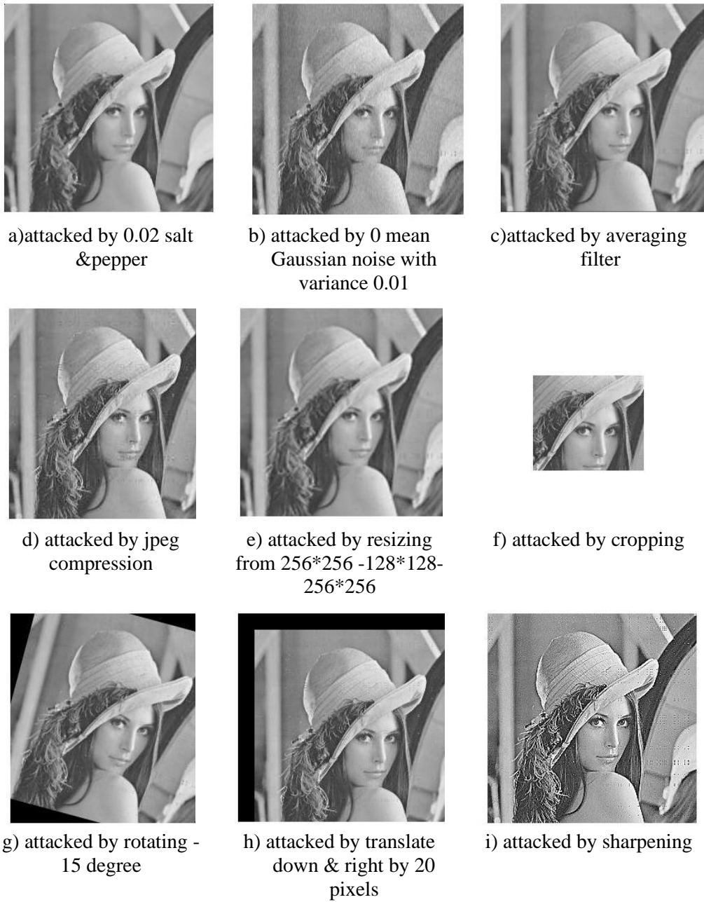
Figure (14) : Watermarked images after attacked by nine types of attacks using FL-EXPW method
