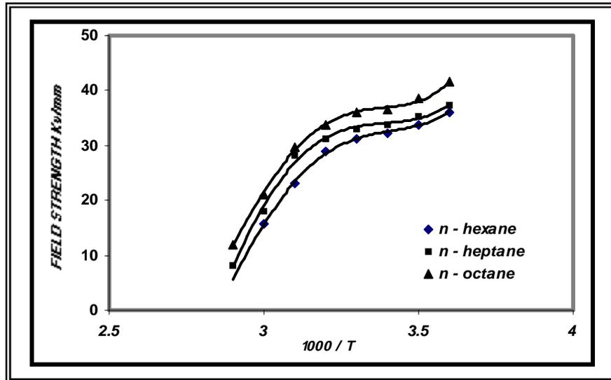
Figure (4) Temperature dependence on breakdown field strength for different saturated hydrocarbon liquids
