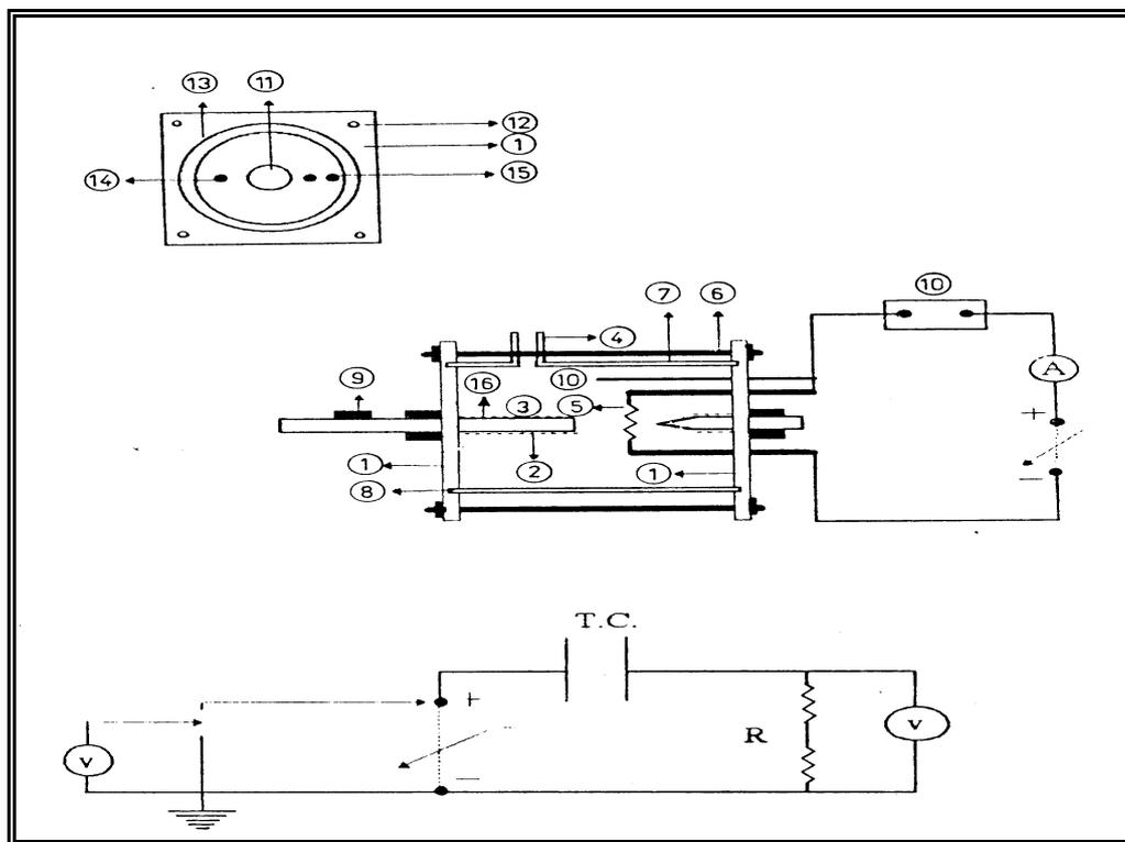
**Figure(1): Experimental apparatus (Schematic diagram of the test cell and electrical circuit. A-Ammeter R-Standard Resistor V-Voltmeter 1-Teflon base 2- Brass needle electrode 3-Brass plane electrode 4-Filling port 5-Heater 6-Steel fitting rod 7-Glass envelop 8-Gasket 9-Brush 10-Temperature control 11-Electrode fitting hole 12-Rod fitting hole 13-Test dell setting grove 14-Heater voltage connection 15-Temperature control hole 16-Insulation cover.**
